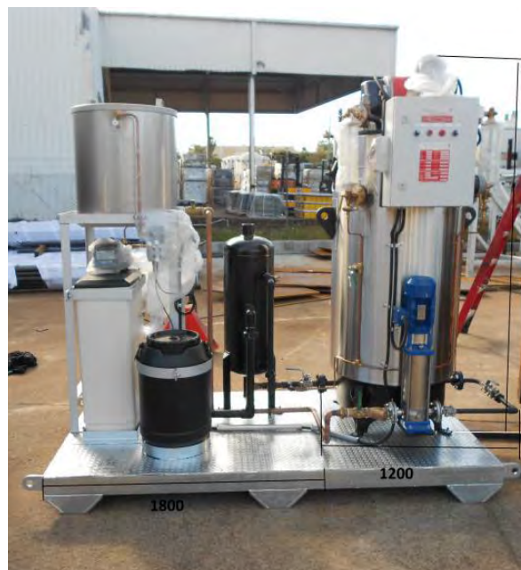
Plate 2-2: LPG fuelled high pressure boiler
