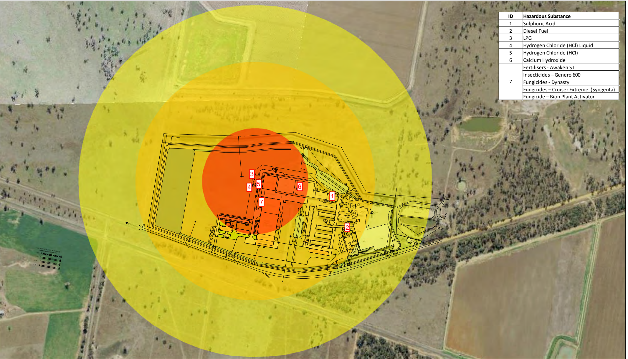
Figure 6-8 Thermal radiation impacts from explosion of LPG tank
